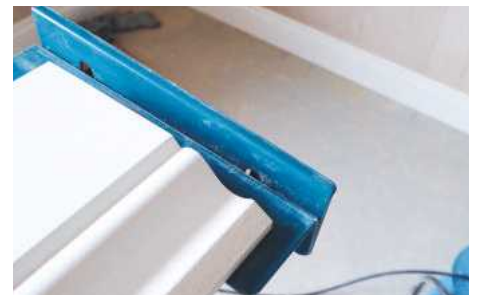
▲ It allows any work to butt up against it for fast repeat cuts
